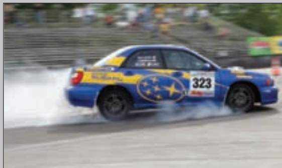
100 percent tire slip, also known as wheel lock, occurs if a vehicle is still moving yet the tire is no longer rotating. This may be amusing for the spectators, but it's not the most effective way to achieve the best possible stopping distance. (Wayne Flynn/pdxsports.com)
